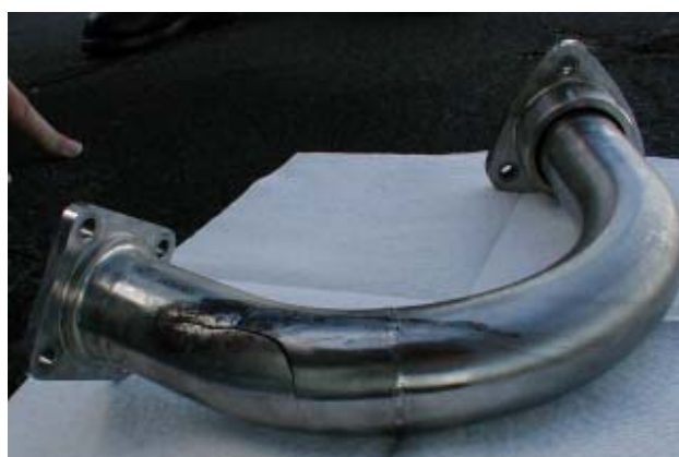
Figure 4 Fuel Pipe Crack & Scratches
